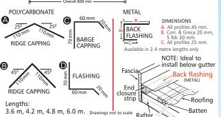
End Closure Foam Strip Anti-noise Tape We recommend the use of self adhesive foam tape on ; RIB – BOTTOM battens to reduce noise created by expansion and contraction of the sheeting.
