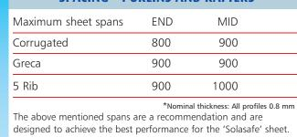
designed to achieve the best performance for the 'Solasafe' sheet Greater spans are possible but may lead to the sheet ocean waving and or water ponding
