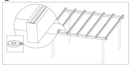
Applying Purlin tape on each rafter will reduce friction and noise.
