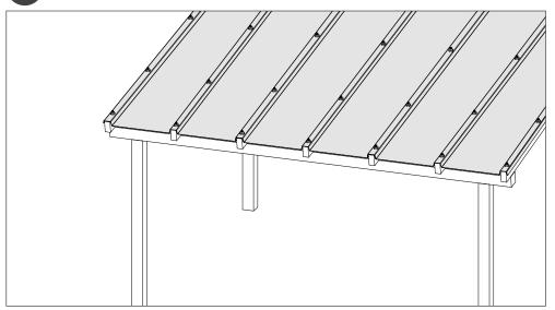
8 Installing Head Wall Flashing (purchased separately)
