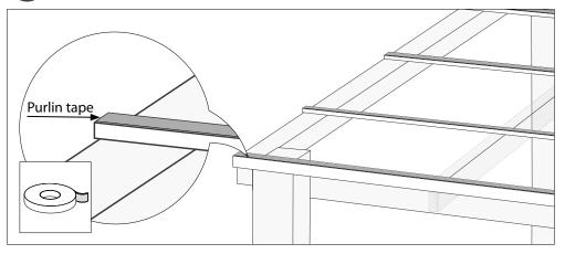
Applying purlin tape on each purlin will reduce friction and noise.
